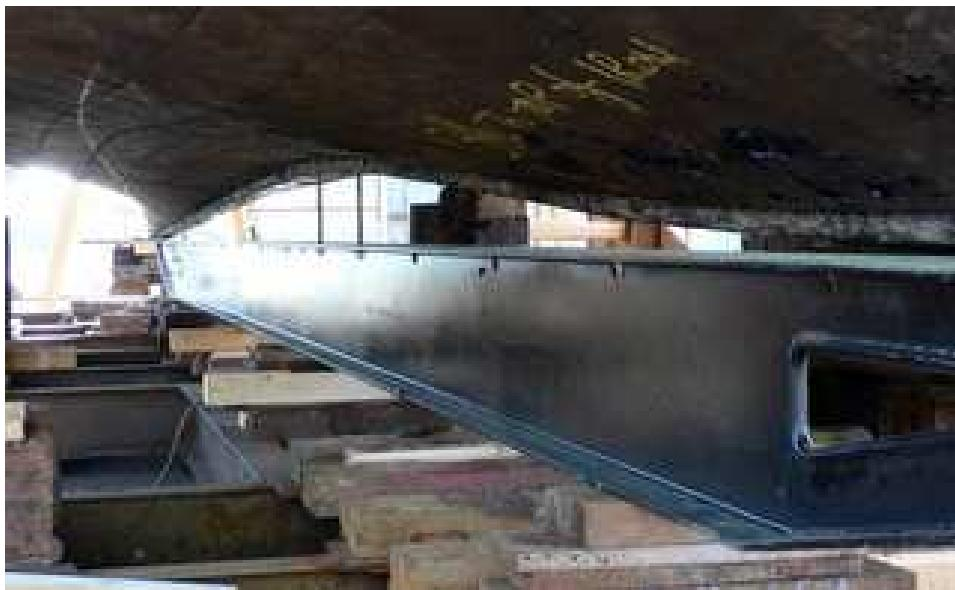
the slip. The procedure was brutally simple. Her old wooden keel was sawn off, old bolts drawn and a template of the new boltholes was fastened to the underside of her hog. All new boltholes were drilled and the new keel/girder was
