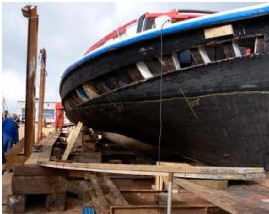
Once on the slip tar was scraped off the hull whilst the boat-builders set about removing the old frames designated for removal on this occasion. As the tar was removed, armed with a drawing board and pencil I produced a schematic of the hull showing the location and length of all planks. This was followed by a condition report on each one ranging from "sound" to "horrendous".
